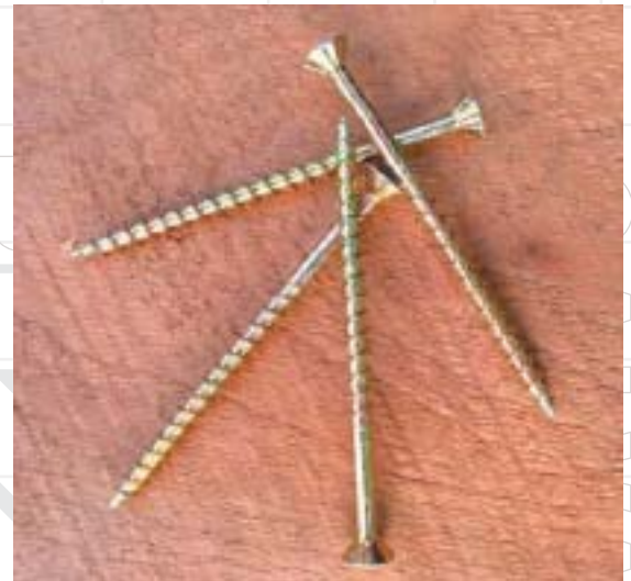
Zinc electroplated coatings are used on a wide range of builders hardware. The relatively thin, pure zinc coating is unsuitable for external applications.
