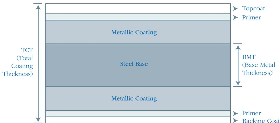
It is important to note that structural capability is a function of base metal thickness and steel grade whereas corrosion performance is afforded by metallic coating thickness and type. Always ensure that the base metal thickness specified is as per recommendations.
