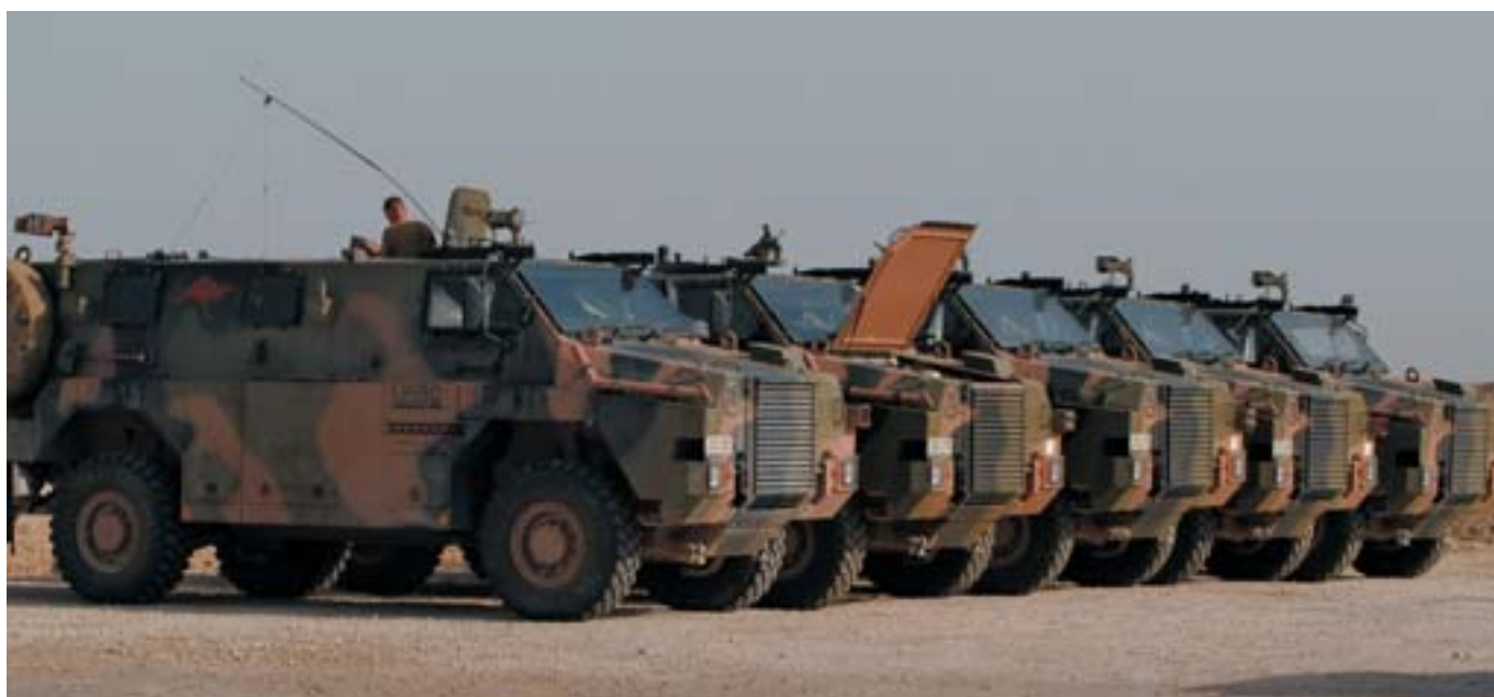
Australian-made Bushmaster protected infantry mobility vehicles which take advantage of high hardness steel plate produced by Bisalloy.
