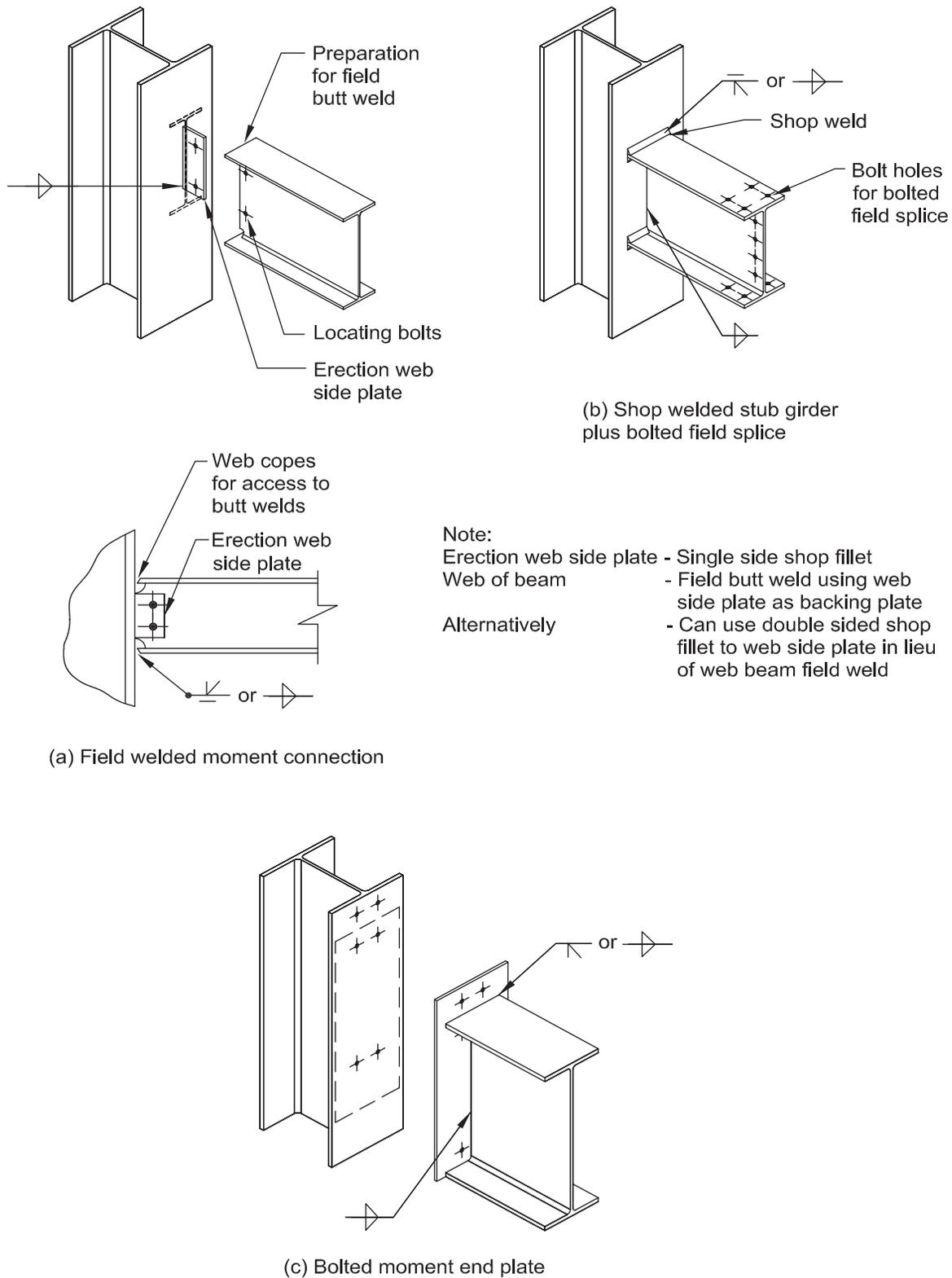
**FIGURE 2. RIGID CONNECTIONS**
