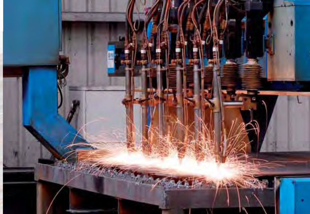
Surdex automated plate cutting in Victoria.
