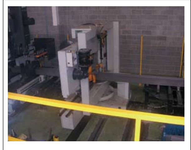
Figure 1: FICEP beam with in-line drill and sawing (Photo courtesy Brian Mahony)
