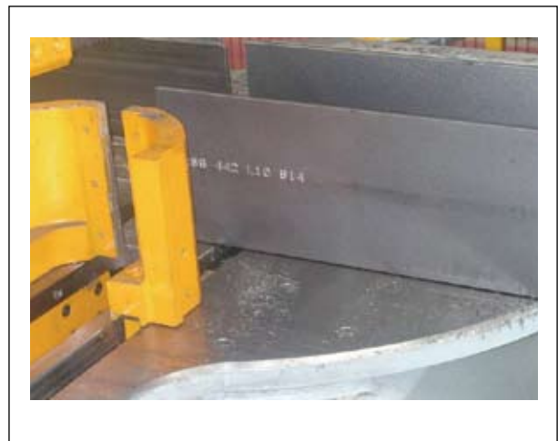
Figure 2: Identification engraved on beam (Photo courtesy Brian Mahony)
