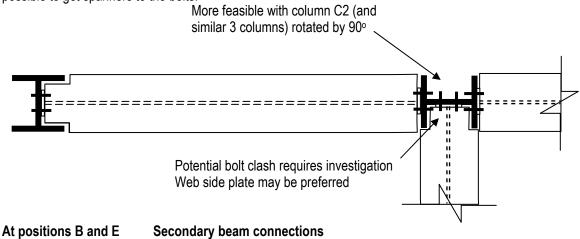
• There is a potential problem with installing all secondary beams as:
