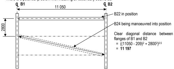
With a clear diagonal distance of 11 197 and the overall length of the beam being  $11\ 050 - 2\ x$  Clearance of 20 mm, this should fit. To confirm this it would be appropriate to set up a 'full scale' CAD drawing model of the assembly and check that the beam can be assembled without snagging on the web cleats to B1 and B2.
