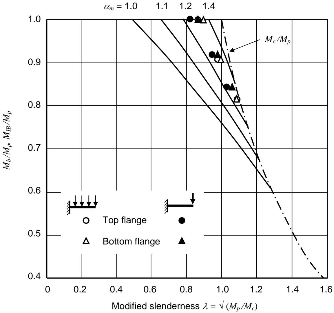
Fig. 7. AISC and Cantilever Strengths by Inelastic Buckling
