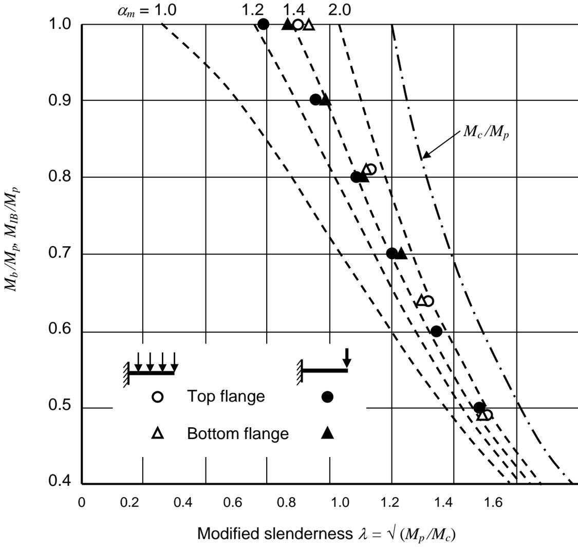
Fig. 5. AS4100 and Cantilever Strengths by Inelastic Buckling
