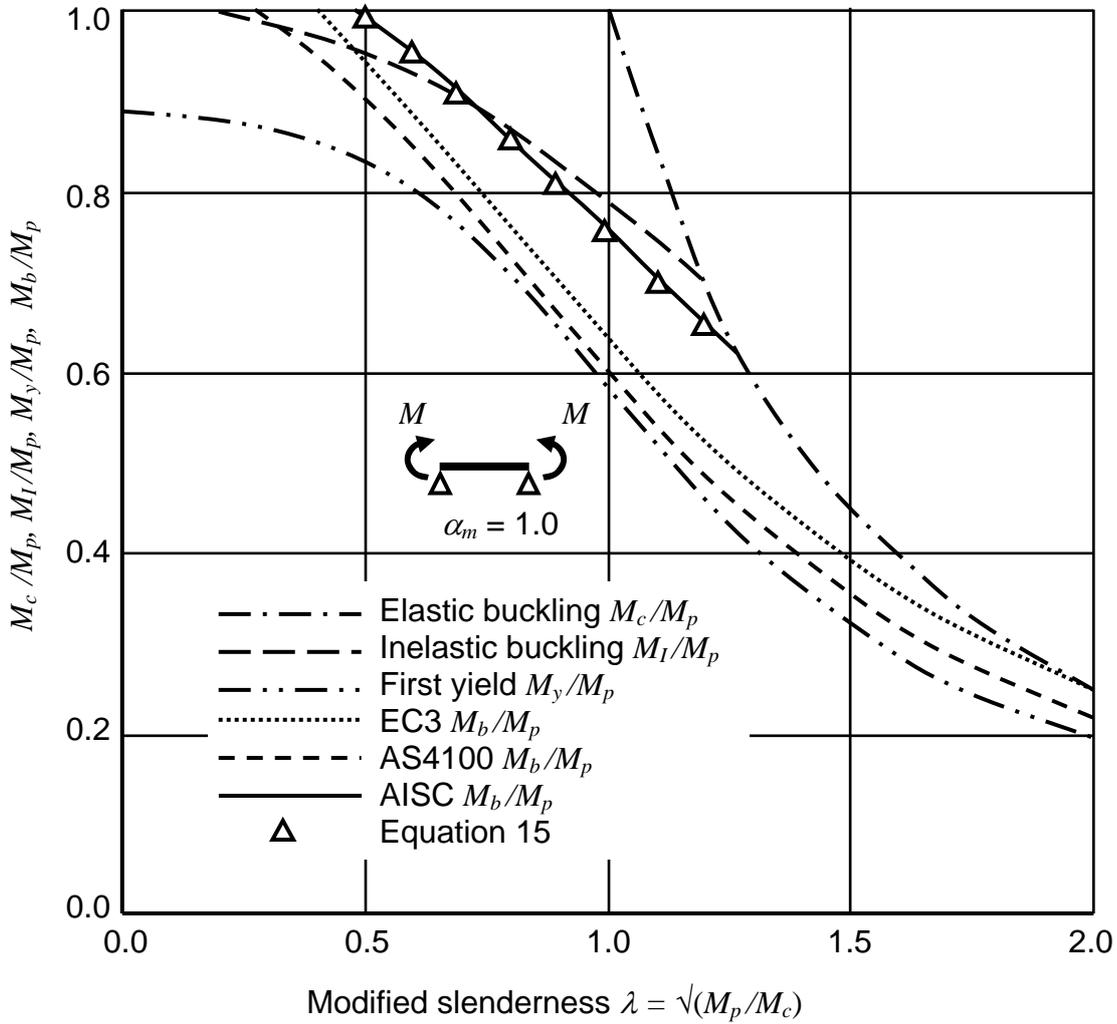
Fig. 3. Buckling, Yielding, and Nominal Design Capacities
