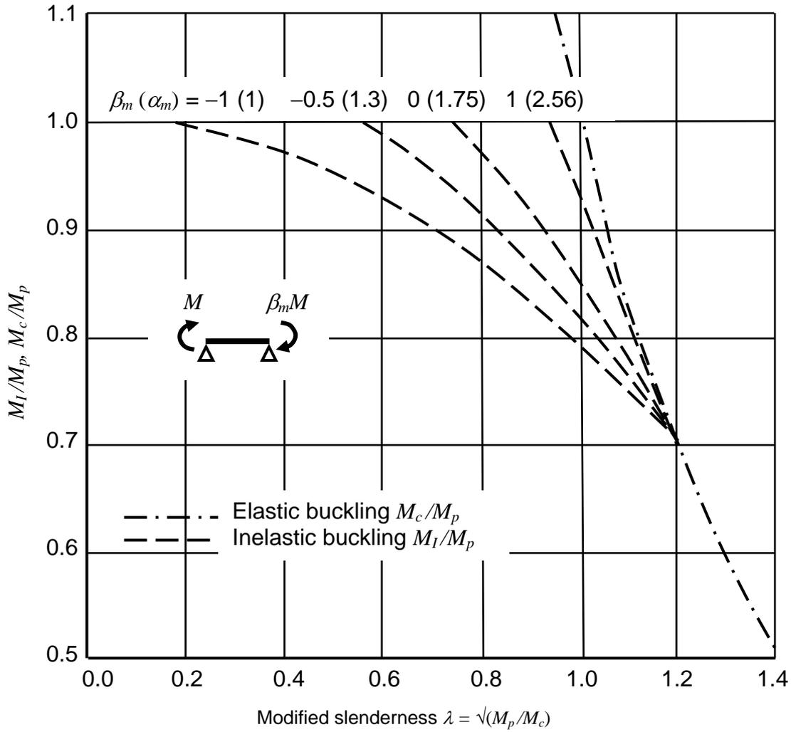
Fig. 2. Inelastic Buckling
