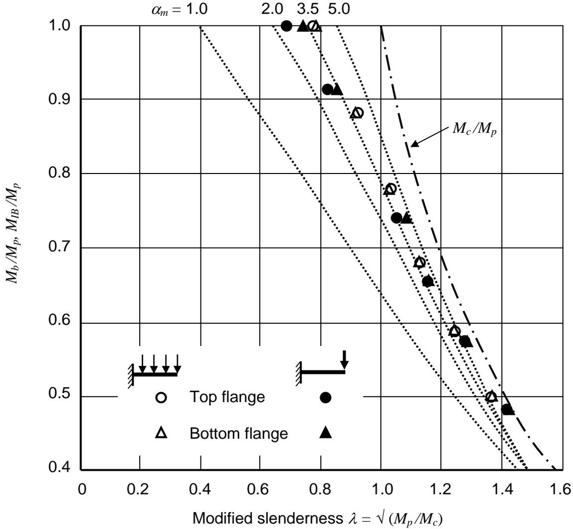
Fig. 4. EC3 and Cantilever Strengths by Inelastic Buckling
