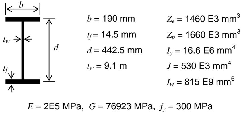
Fig. 6. Section Properties
