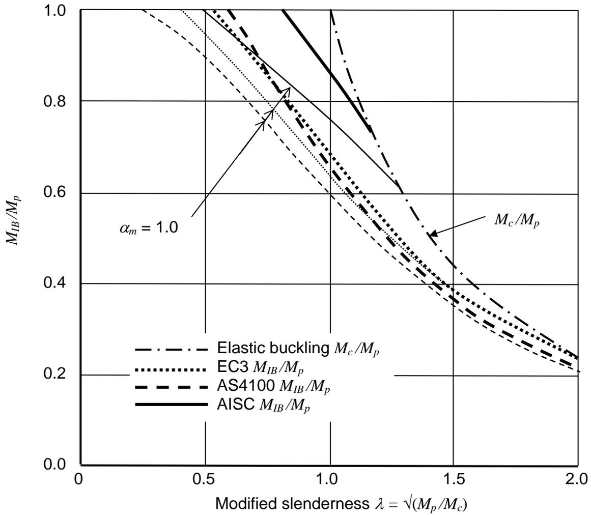
Fig. 10. Example Nominal Design Strengths
