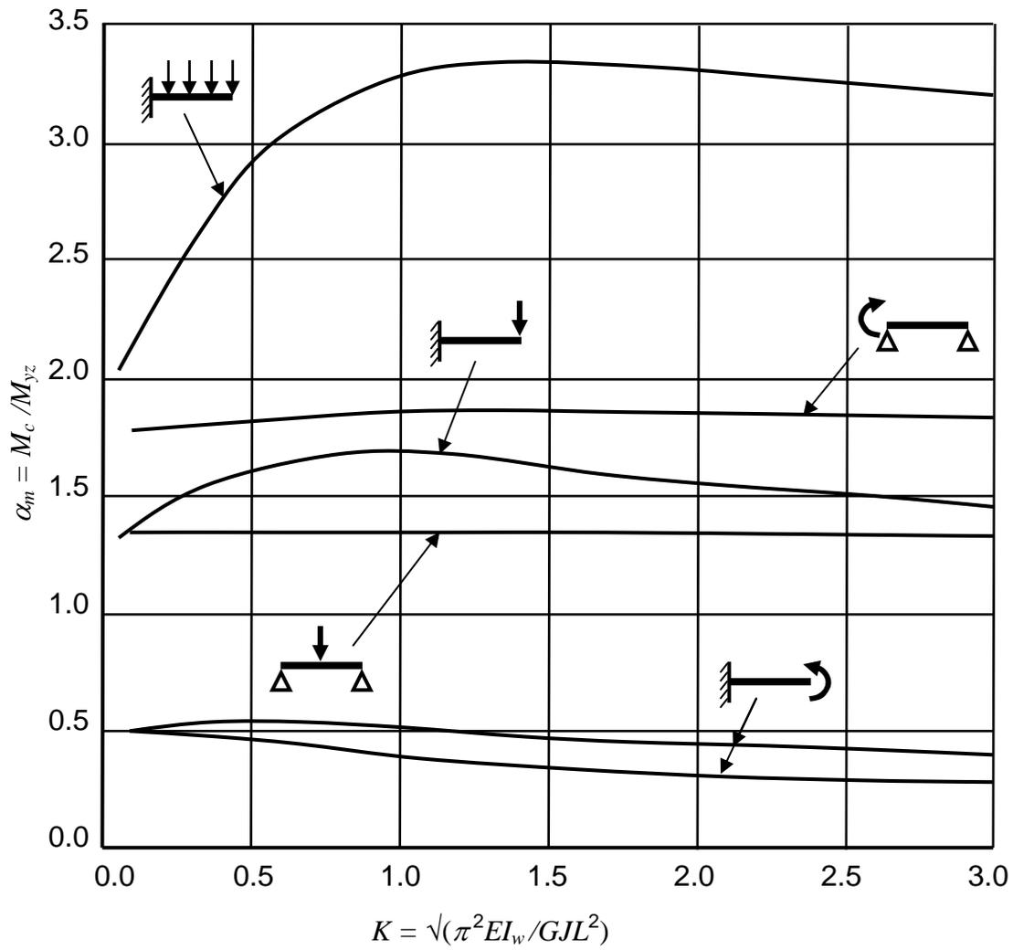
Fig. 1 Elastic Buckling Values of  $\alpha_m$
