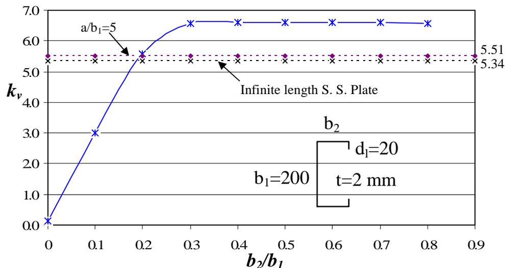
Figure 1. The Ratio of Flange and Web Widths ( $b_2/b_1$ ) and The Shear Buckling Coefficients ( $k_v$ )
