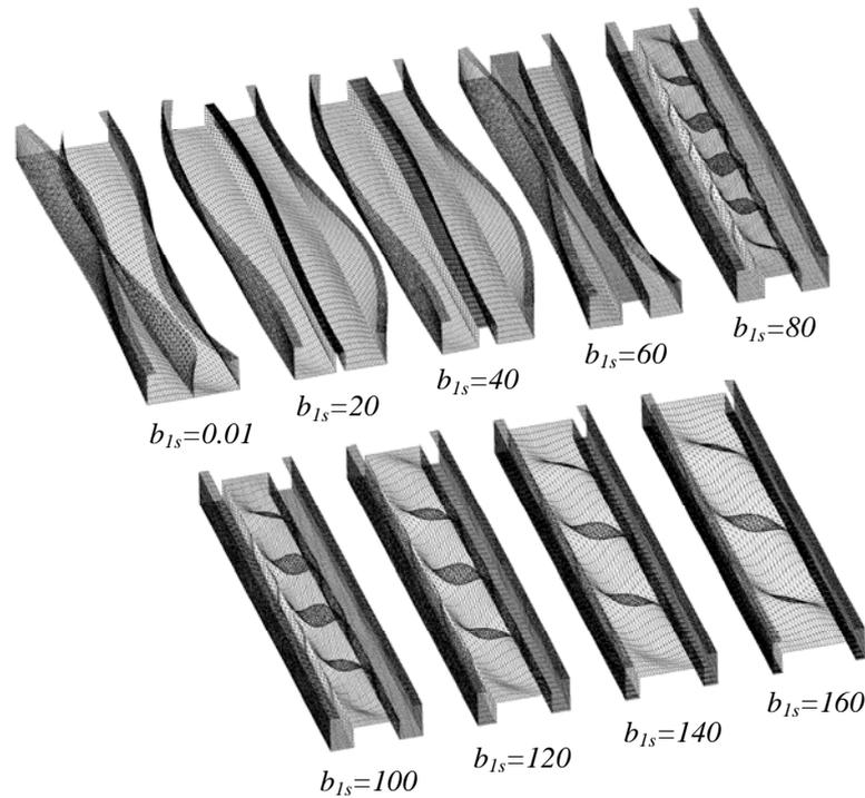
Figure 8. Buckling Mode Shape of Lipped Channel Section with Intermediate Web Stiffener –  $b_{2s} = 50$  mm
