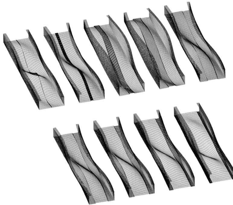
Figure 7. Buckling Mode Shape of Lipped Channel Section
