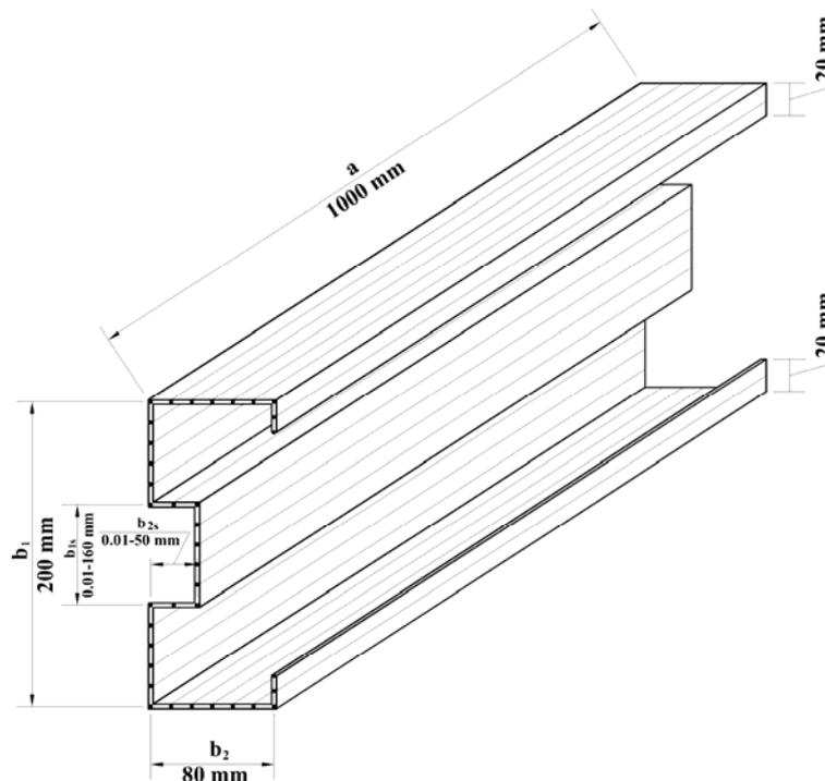
Figure 3. Lipped Channel Geometry with an Intermediate Stiffener
