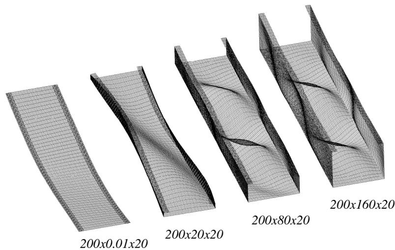
Figure 2. Buckling Mode Shape of Lipped Channel Section – Length = 1000 mm,  $a/b_1=5$
