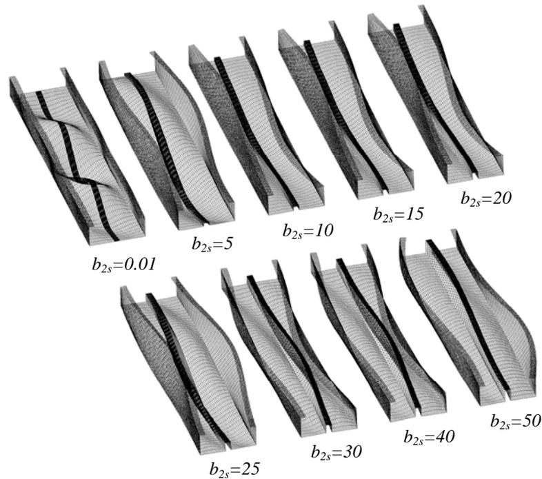
Figure 10. Buckling Mode Shape of Lipped Channel Section
