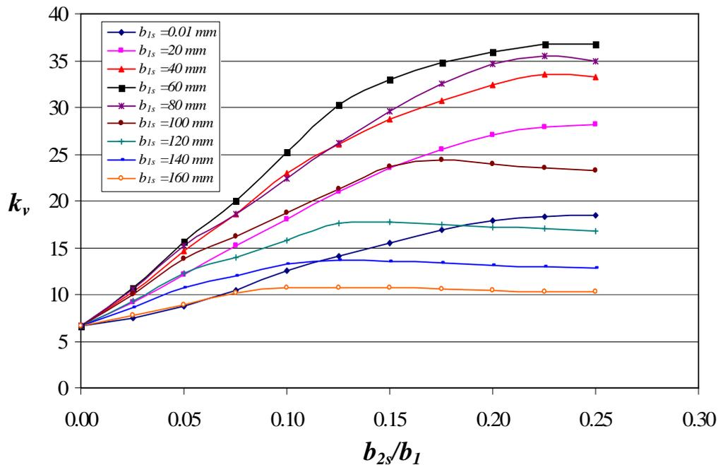
Figure 9. The Ratio of Stiffener Widths and Web Widths ( $b_{2s}/b_1$ ) and The Buckling Coefficients ( $k_v$ ) Of Lipped Channel Section with Intermediate Web Stiffener
