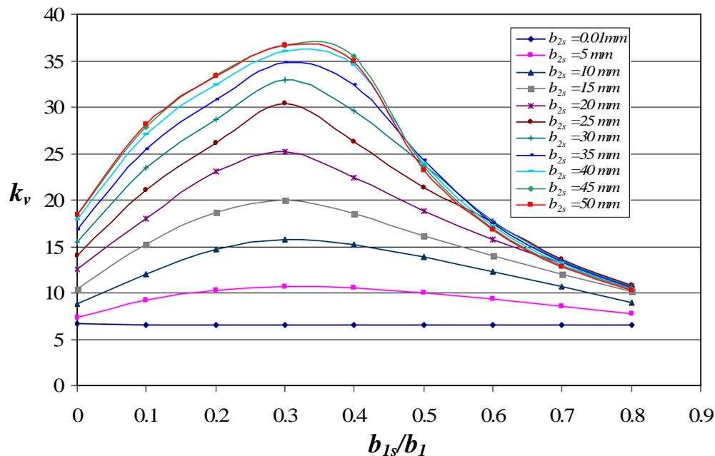
Figure 6. The Ratio of Stiffener Depths and Web Widths ( $b_{1s}/b_1$ ) and The Buckling Coefficients ( $k_v$ ) Of Lipped Channel Section with an Intermediate Web Stiffener
