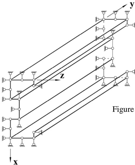
Figure 5. Boundary Conditions of Lipped Channel with an Intermediate Web Stiffener
