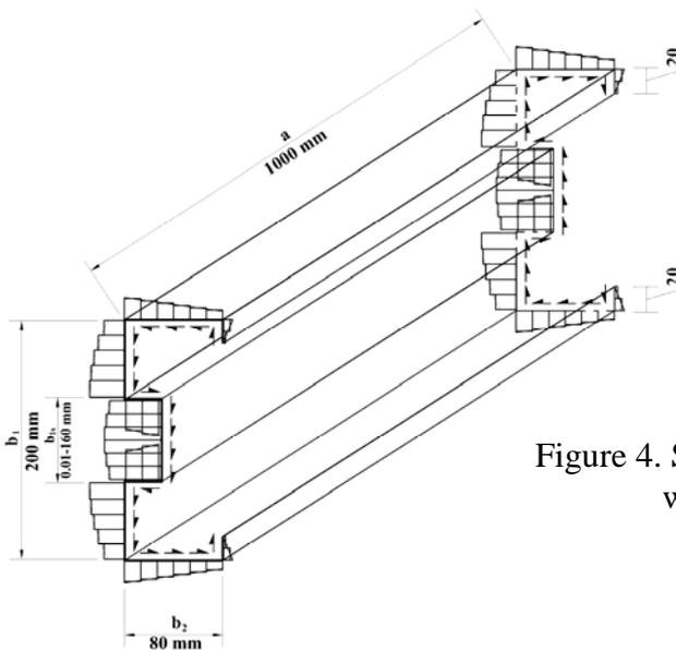
Figure 4. Shear Flow Distribution in Lipped Channel with an Intermediate Web stiffener
