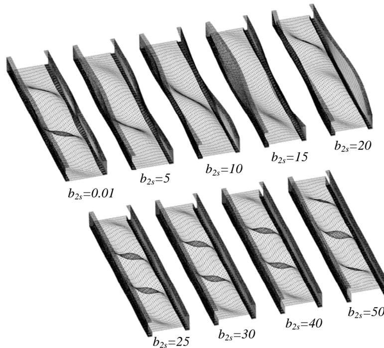
Figure 11. Buckling Mode Shape of Lipped ChanWel Section with Intermediate Web Stiffener –  $b_{1s} = 160 \text{ mm}$
