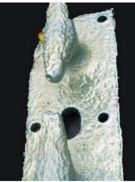
This 50-year old cast marine bollard has been hot dip galvanized. Although it is badly pitted, the bollard was easily re-galvanized to restore its durability.
