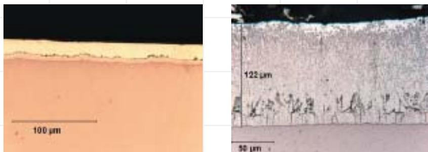
*These two micrographs illustrate the difference between a continuously galvanized coating (l) and a hot dip galvanized coating (r) The continuously galvanized coating is almost 100% zinc while the hot dip galvanized coating, as well as being significantly thicker (122 microns versus 20 microns) is almost 100% zinc-iron alloy.*
