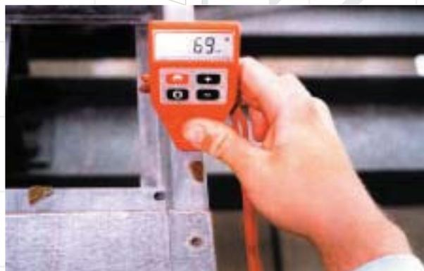
*The Orica petrochemical plant at Port Botany, Sydney was galvanized in 1977. Thickness testing of the galvanized coating after 25 years indicated that the coating has a remaining service life exceeding 30 years, with nearly 70 microns of coating remaining of the original 100 microns.*
