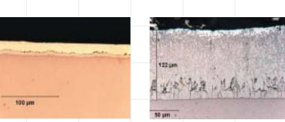
These two micrographs illustrate the difference between a continuously galvanized coating (I) and a hot dip galvanized coating (r) The continuously galvanized coating is almost 100% zinc while the hot dip galvanized coating, as well as being significantly thicker (122 microns versus 20 microns) is almost 100% zinc-iron alloy.
