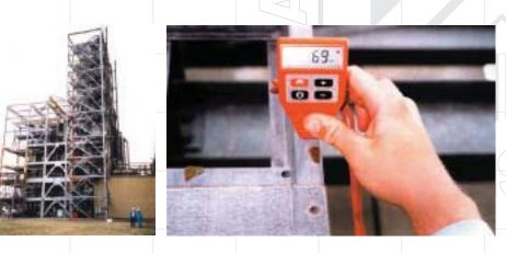
The Orica petrochemical plant at Port Botany, Sydney was galvanized in 1977. Thickness testing of the galvanized coating after 25 years indicated that the coating has a remaining service life exceeding 30years, with nearly 70 microns of coating remaining of the original 100 microns.
