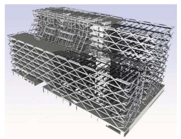
Following completion of the structure and removal of all building formwork the columns were then jacked up and bolted to the truss, which then withstood the permanent building load of floors the building. six of Following the completion of this the temporary columns were removed, reinstating full access to the basements.
