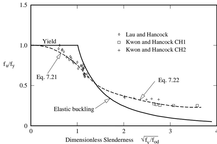
**Fig. 7.5 Distortional buckling strength design curves for compression**
