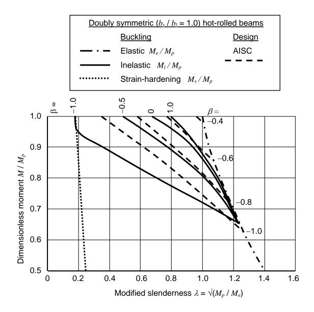
Fig. 8 Inelastic Buckling Under Moment Gradient
