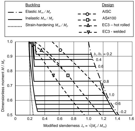
Fig. 5 Inelastic Buckling of Welded Beams - Uniform Bending
