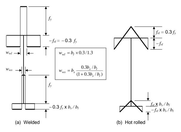
Fig. 3 Residual Stresses in Monosymmetric Beams
