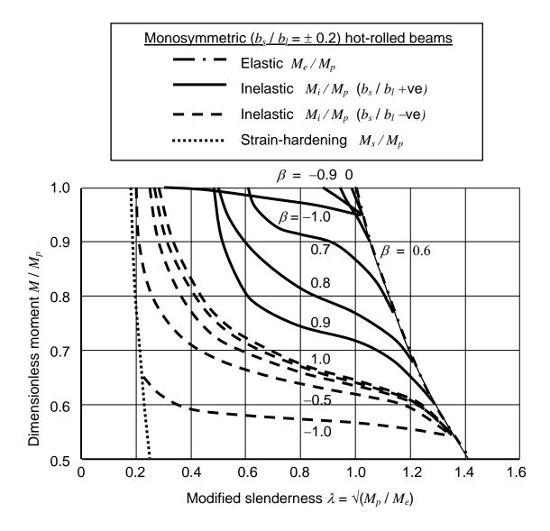
Fig. 10 Inelastic Buckling Under Moment Gradient
