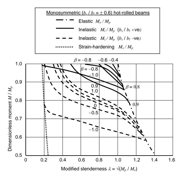
Fig. 9 Inelastic Buckling Under Moment Gradient
