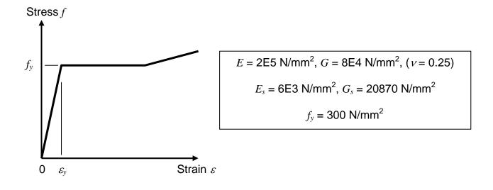
Fig. 2 Material Properties of Monosymmetric Beams
