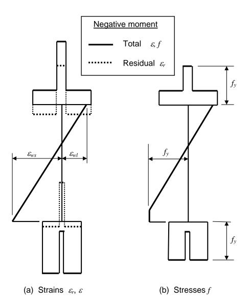
Fig. 4 Total Strains and Stresses in Welded Beams
