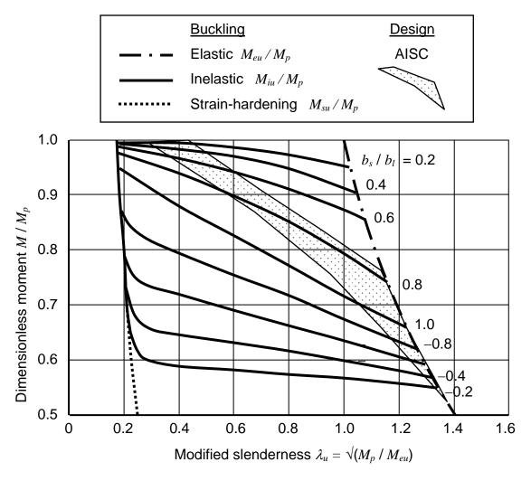
Fig. 6 Inelastic Buckling of Hot Rolled Beams – Uniform Bending
