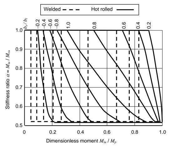
Fig. 7 Inelastic Stiffnesses of Monosymmetric Beams
