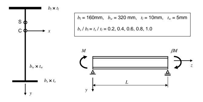
Fig. 1 Geometry and Loading of Monosymmetric Beams
