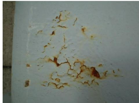
Figure 4: Poor paint finish
