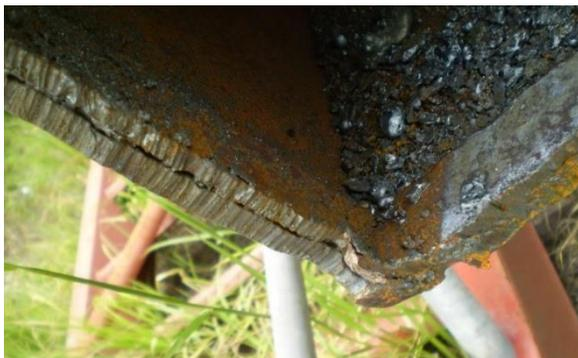
Figure 3: Fillet welded connection instead of butt weld
