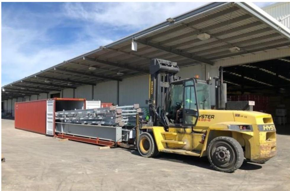
*Figure 9: Imported welded 3 plate beams being unloaded from a shipping container*
