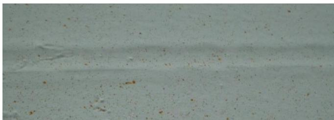
Figure 5: Under-cut (concave) weld below required thickness
