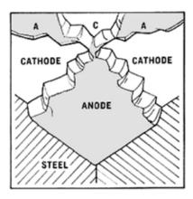
As anode areas corrode new material of different composition and structure is exposed. This results in changes in electrical potentials, causing anodes and cathodes to exchange roles, though not all at once, and areas previously uncorroded are now attacked. These processes may continue until the steel is entirely consumed.
