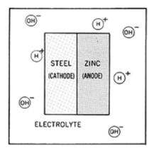
As a result of the differences in electrical potential within the cell, negatively charged electrons flow from the zinc anode to the steel cathode and zinc atoms in the anode are converted to positively charged zinc ions.
