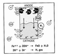
Under suitable conditions corrosion occurs at the rate of billions of complete reactions every second and soon results in a layer of rust appearing over the surface of the anode area.
