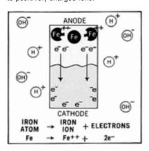
The positively charged iron ions of the anode attract and react with negatively charged hydroxyl ions in the electrolyte to form iron oxide or rust. Negatively charged electrons react at the cathode surface with positively charged hydrogen ions in the electrolyte to form hydrogen gas.
