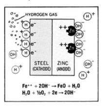
When discontinuity or damage in the zinc coating exposes the underlying steel, the cathodic protection which zinc provides for steel comes into action and ensures that the exposed steel does not corrode.
