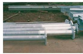
**Double dipping** or galvanizing a second time will not increase the thickness of a galvanized coating for reasons discussed under "Coating thickness", and may adversely affect coating appearance.
