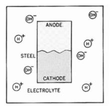
As the result of differences in electrical potential within the cell, negatively charged electrons flow from anode to cathode and iron atoms in the anode area are converted to positively charged ions.
