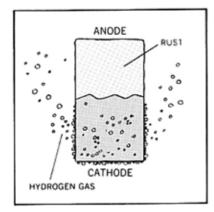
The anode and cathode areas on a piece of steel are actually microscopic. When greatly magnified the surface might appear as the mosaic of anodes and cathodes visualised here, all electrically connected by the underlying steel. Corrosion occurs in the anode areas.
