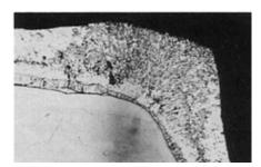
Galvanized coatings are slightly thicker at corners and edges as shown, an important advantage over most organic coatings which thin out in these critical areas.
