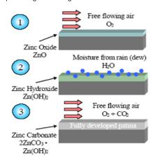
The zinc patina begins its development with exposure to oxygen in the atmosphere. Moisture from rain or humid air reacts with this layer to form zinc hydroxide. This layer then reacts with carbon dioxide present in the atmosphere to form the tightly adherent, insoluble zinc patina.
