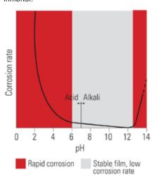
In the range pH 6 to pH 12.5 the zinc coating forms a stable protective film and corrosion rate is low.
