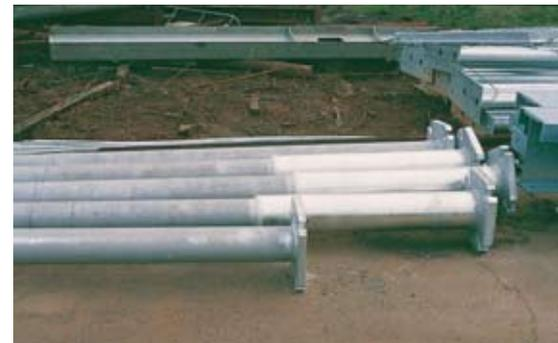
**Double dipping** or galvanizing a second time will not increase the thickness of a galvanized coating for reasons discussed under "Coating thickness", and may adversely affect coating appearance.
