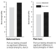
Pull-out testing showed no significant difference in bond strengths, due to the effect of mechanical interlock. Tests showed no significant effect of chromate additions on the bond strength of deformed galvanized bars. Bond strengths of galvanized plain bars at various levels of chromate additions to concrete\*
