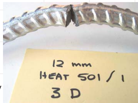
Micro-alloyed 12 mm 500n Grade reinforcing bar failed rebend testing around 3D radius
