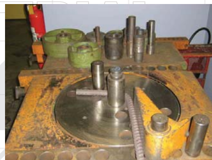
500N Grade reinforcing bar presents no problems if galvanized after bending if AS3600 standards are complied with in the processing
