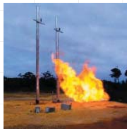
CSIRO Bushfire CRC – Mogo NSW. Sureline galvanized steel poles undergoing Level 2 bushfire testing. This test simulates actual bushfire conditions and flame duration. Galvanized coating unaffected.
