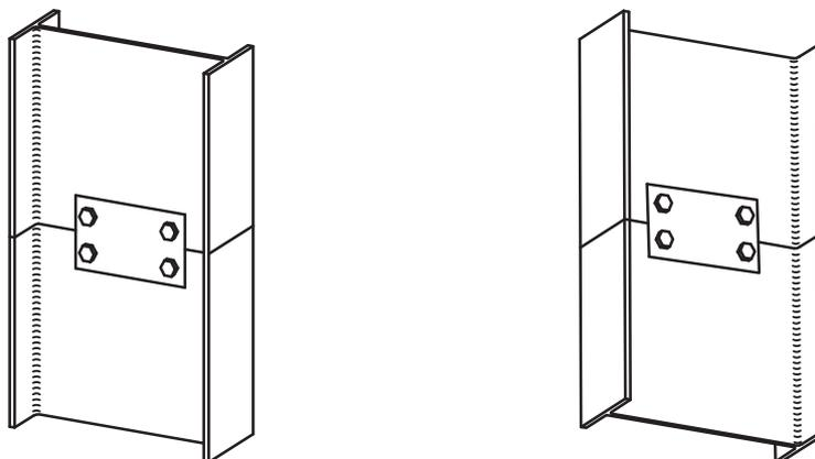
FIGURE 48 FULLY WELDED SPLICE
