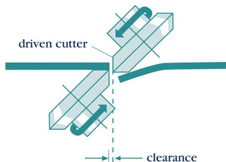
As with straight blade shearing, selection of correct clearance is necessary to obtain optimum edge quality and cutter life. Negative clearance,
