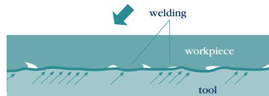
(c) Normal and shear loading leading to further flattening distortion, and welding with tearing
