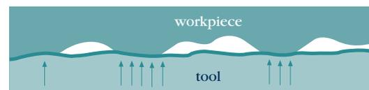
(a) Light normal loading of unlubricated surfaces
