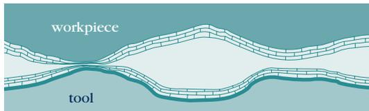
(c) Extreme pressure boundary lubrication with a pigment (mechanical EP agent)
