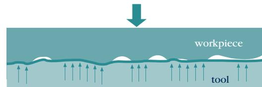
(b) Heavier normal loading with asperity flattening
