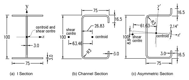
Figure 7 Dimensions for I, channel and asymmetric sections (in mm)
