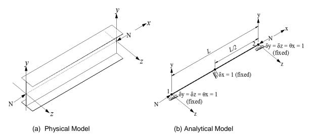
Figure 8 I-section column subjected to compressive load
