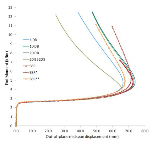
Figure 14 End moment vs out-of-plane midspan displacement for I-beam in major axis bending
