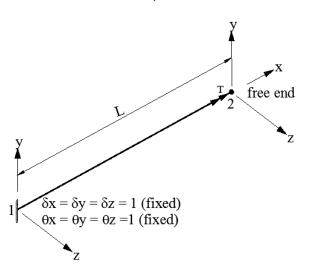
Figure 22 Cantilever channel beam subjected to torsion at the free end
