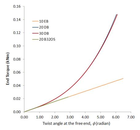
Figure 23 Torsional response of channel beam
