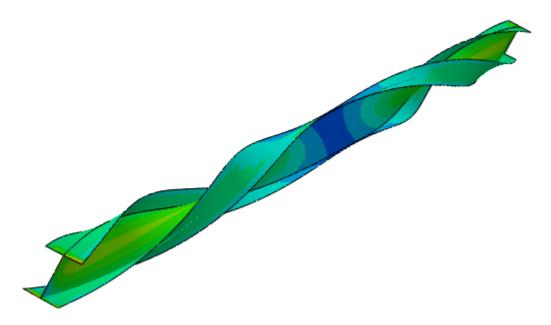
Figure 10 Final deformed state of I-section column ( $\phi$ =206°)
