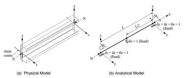
Figure 16 Channel column subjected to compression
