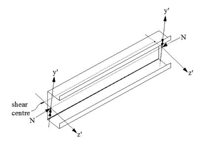
Figure 24 Asymmetric section column subjected to axial compression
