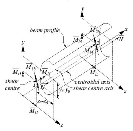
Figure 5 Element force system with axial force acting at the centroid
