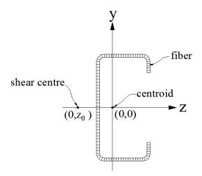
Figure 6 Fiber representation of channel section
