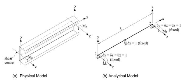
Figure 18 Channel beam subjected to major axis bending
