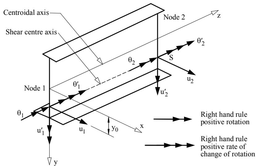
(a) Nodal displacements producing out-of-plane deformation
