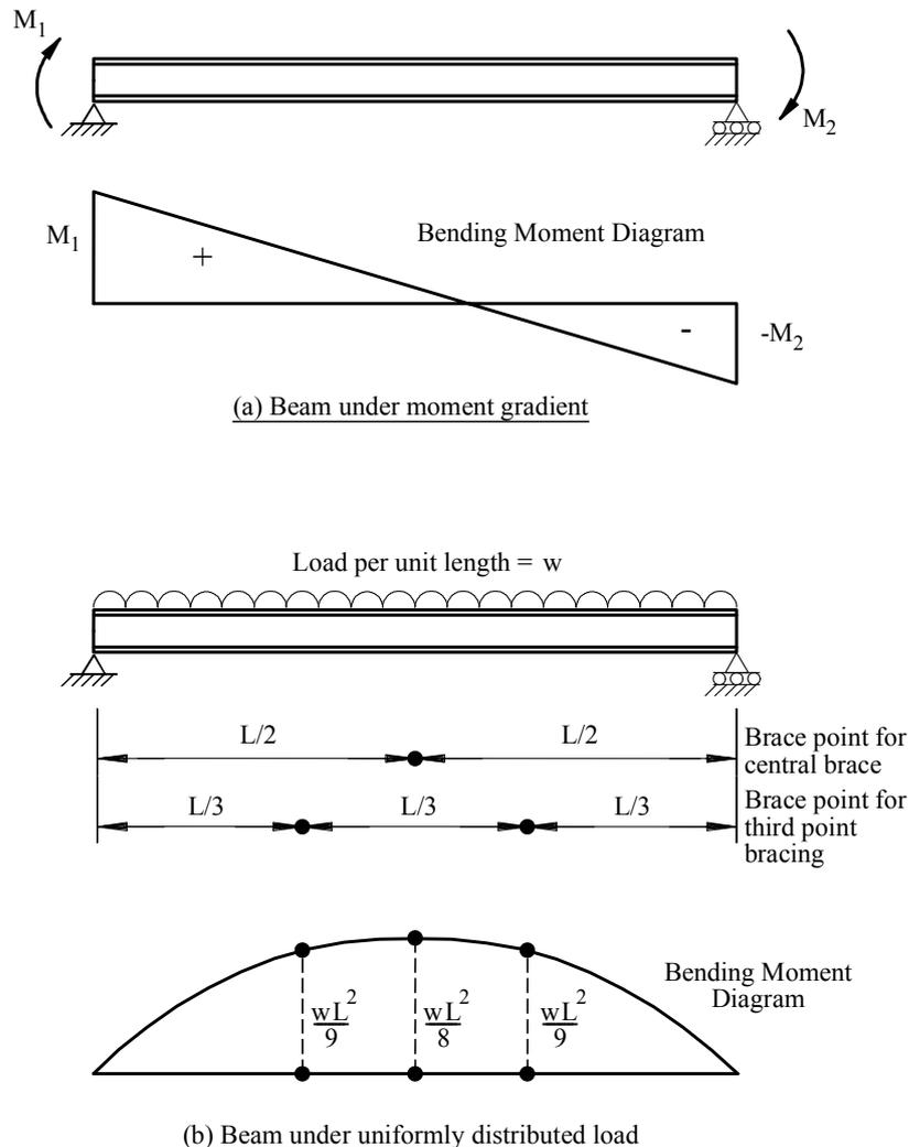
**Fig. 5.2 Simply supported beams**
