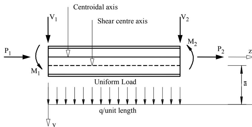
(b) Element actions in the plane of the structure
