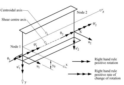
(a) Nodal displacements producing out-of-plane deformation
