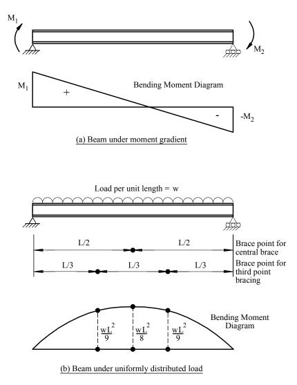
Fig. 5.2 Simply supported beams
