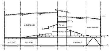
the building, principally some of the primary beams and columns within the promenade area adjacent to and providing direct support to the cinemas. A cross-section showing the promenade in relation to the seating tiers is shown above.
