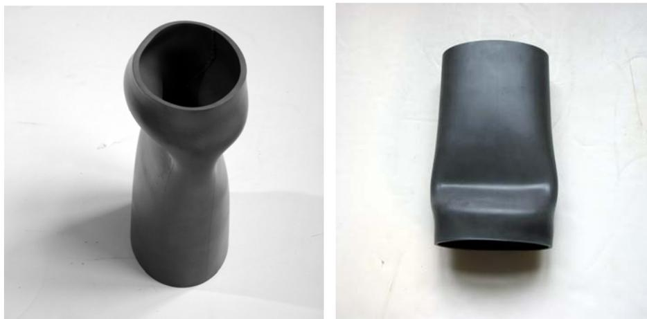
Figure 12. Deformed Shape of Specimen from Tests
