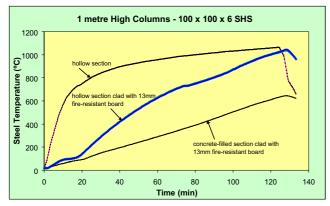
It can be seen that the presence of concrete filling greatly increases the fire-resistance of an externally protected member over that associated with an identical member that is not concrete-filled. The reduction in steel temperature due to concrete filling is only apparent for externally protected members¹.
