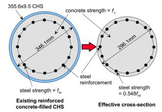
The strength of the column with the effective cross-section can be assessed in accordance with AS3600[23].
