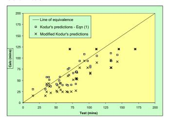
It can be seen that there is a correlation between the predicted fire resistances and those obtained from the tests. If the formula (Eqn (1)) predicted exactly the fire resistance obtained from the tests then all of the points would fall along the line of equivalence. About one half of the points fall above the line.
