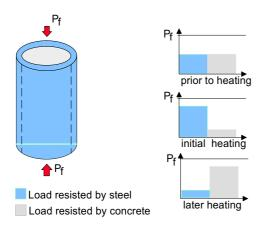
It is the ability of the concrete core to carry load when the steel tube cannot that is the main benefit provided by concrete filling.
