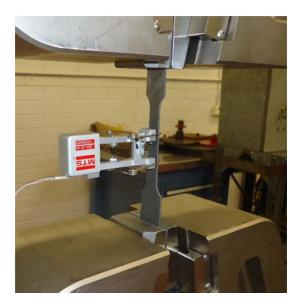
Figure 4. Coupon test configuration
