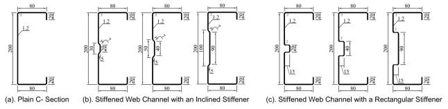
Figure 2. Stiffened web channel types
