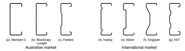
Figure 1. Profile shapes of manufactured purlin profiles
