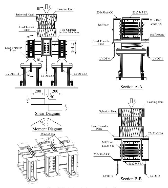
Figure 5: Predominantly shear test configuration
