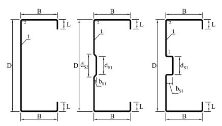
Figure 3. Cross section geometries
