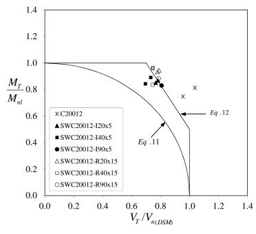
**Figure 9**: Interaction between  $(M_T/M_{nl})$  and  $(V_T/V_{n(DSM)})$
