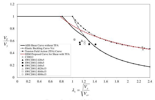
Figure 8: Test data vs DSM shear curves
