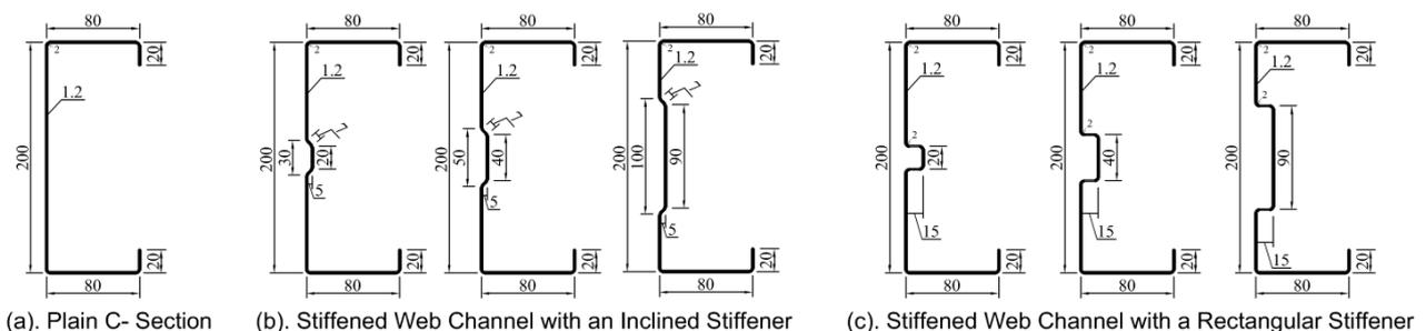
Figure 2. Stiffened web channel types
