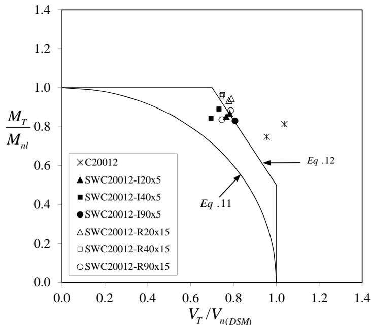
**Figure 9:** Interaction between  $(M_T/M_{nl})$  and  $(V_T/V_{n(DSM)})$
