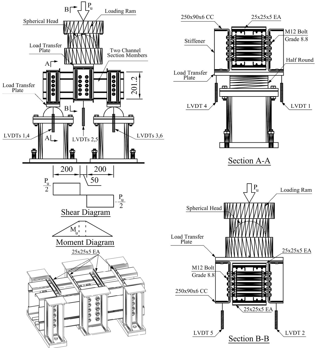
**Figure 5:** Predominantly shear test configuration
