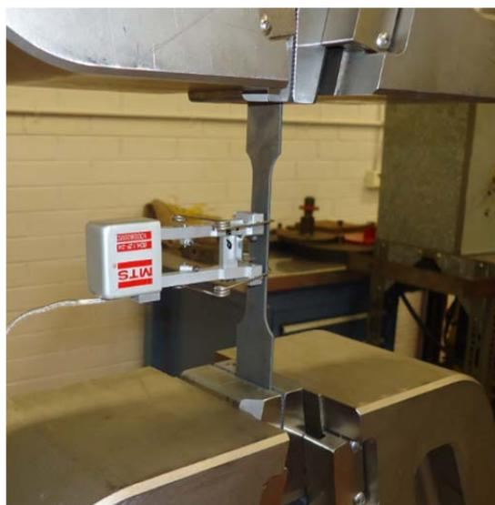
Figure 4. Coupon test configuration
