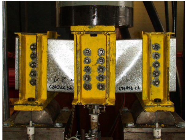
Figure 40. V Test Series Buckling Mode Shape
