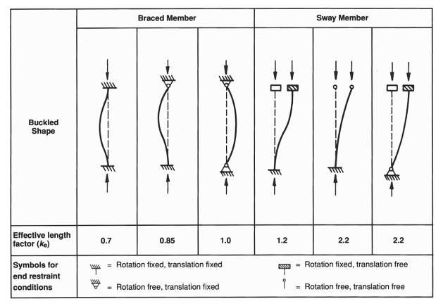
Figure 6.1: Effective Length Factors for Members with Idealised Conditions of End Restraint (Figure 4.6.3.2 of AS 4100)
