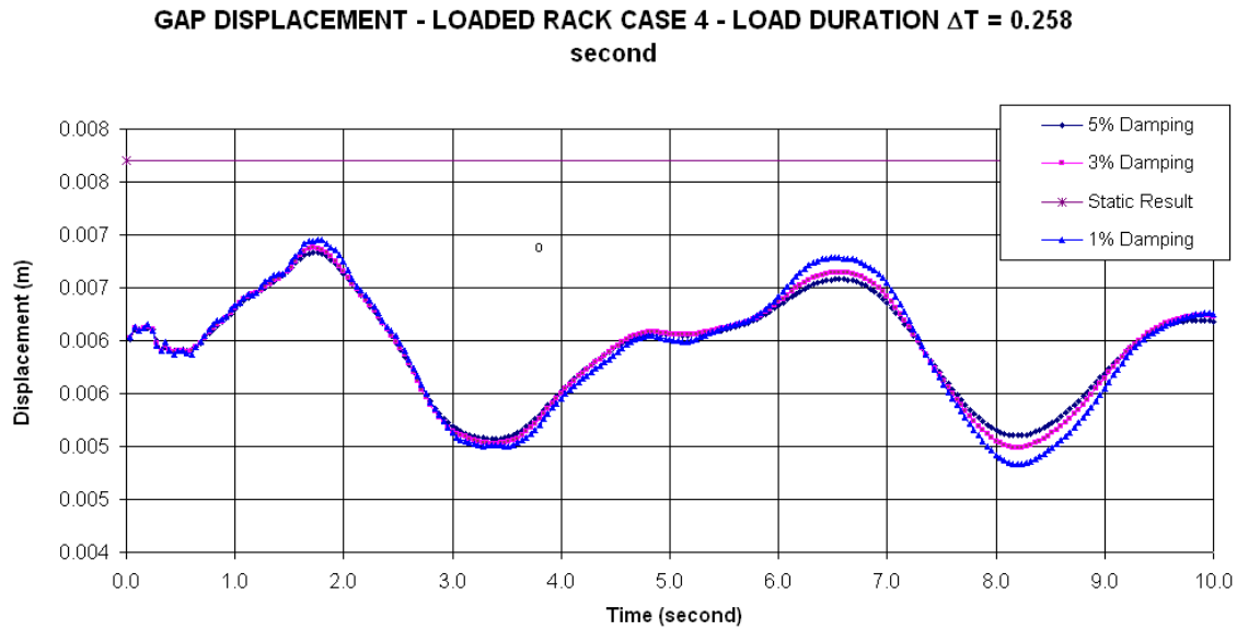
Figure 12i. Displacement Gap Response at the front face of top pallet level – Loaded Rack Case 4 – Load Duration \Delta T = 0.258 second
