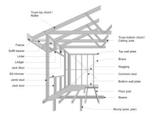
Figure 2: Structural components of typical residential and low-rise structure [7]
