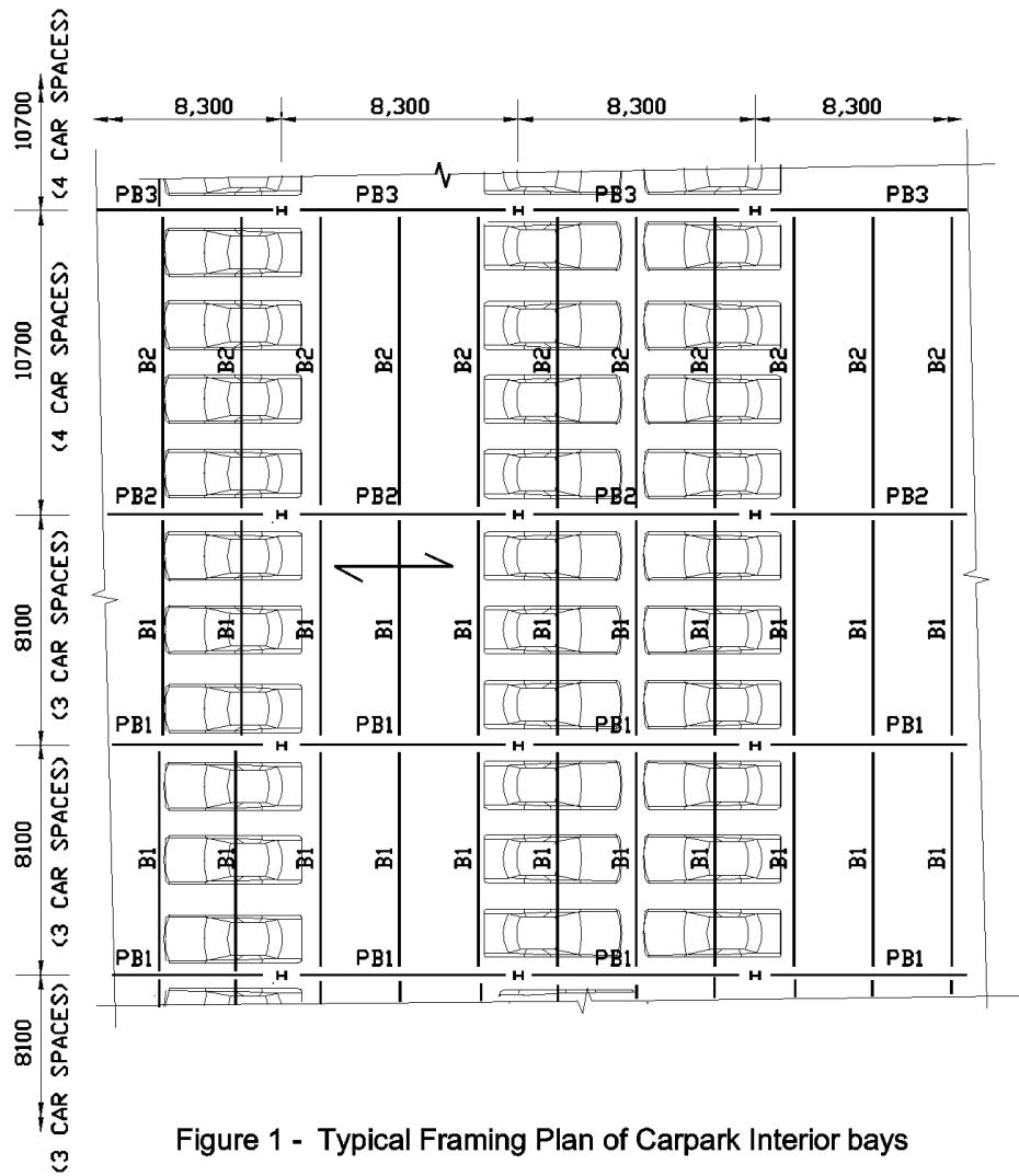
Figure 1 - Typical Framing Plan of Carpark Interior bays
