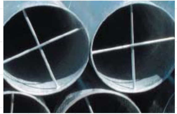
The cross bracing in this tin-walled spiral welded pipe prevents the ends from sagging under their own weight during galvanizing.
