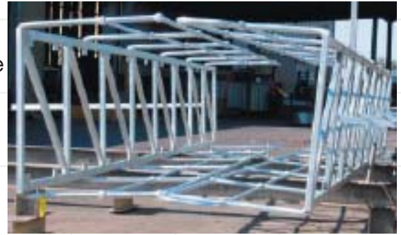
3-D fabrications made up of complex hollow sections require careful design detailing to ensure they can be successfully hot dip galvanized, because of the venting and draining requirements of the individual elements.
