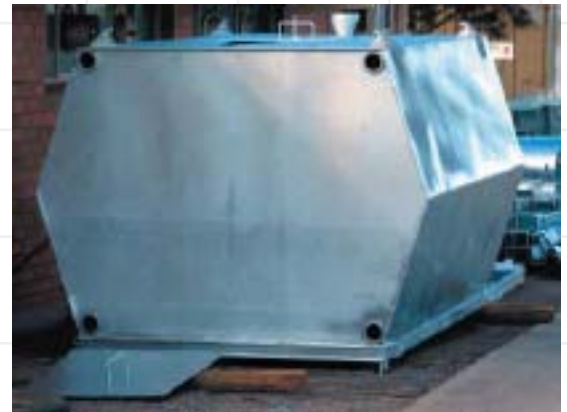
Large hollow vessels such as this water tank require large vent and drain holes to ensure that molten zinc can flow in and out. A tank of this size would hold nearly 15 tonnes of molten zinc.
