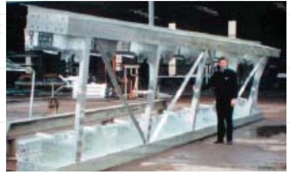
Large fabrications can be galvanized by double-end dipping as long as they do not exceed galvanizing bath size in two dimensions.
