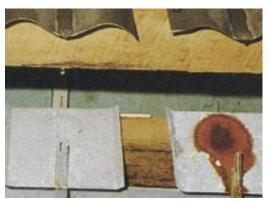
**Test 3:** ZINCALUME<sup>®</sup> steel to ZINCALUME<sup>®</sup> steel gutter (*left*); ZINCALUME<sup>®</sup> steel to zinc-coated steel gutter (*right*).
