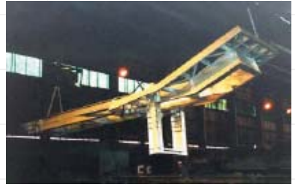
Fabrications like this large frame require double dipping, which is typically 30% higher cost than single dipping because of the extra time in handling.
