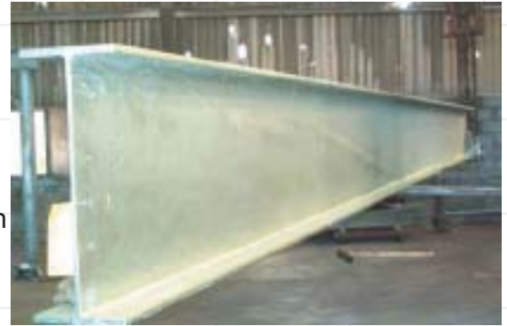
Large and simple structural members such as this universal beam can be galvanized at lower cost because of the ease of handling, the significant mass and relatively low zinc pick up on the heavy section.
