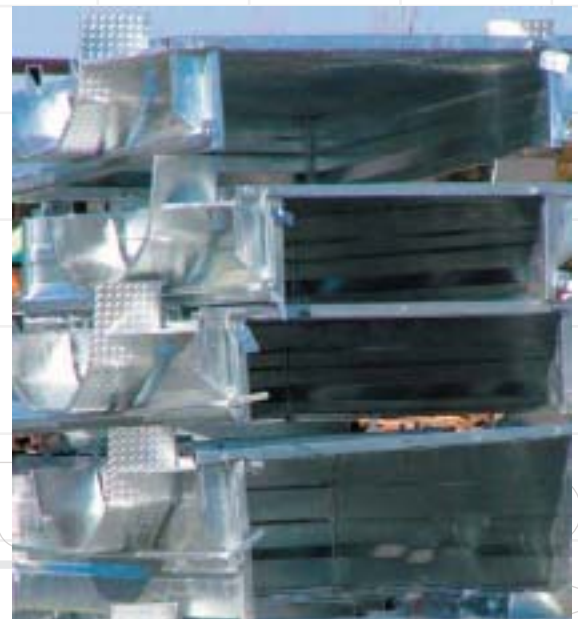
Box trailers have a very high surface area per tonne (about 200 m 2 ) and have a low mass compared to their volume, dictating a relatively high galvanizing cost per tonne but a low coating cost per m 2 .
