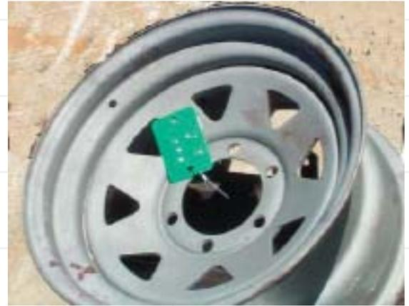
*Items are individually tagged for identification. The metal tag remains attached throughout the galvanizing process.*
