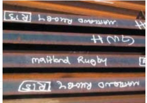
*Clearly marked items make processing of loads easier for both client and galvanizer. The correct type of strippable marking paint should be use to ensure removal in the pre-treatment process prior to galvanizing.*
