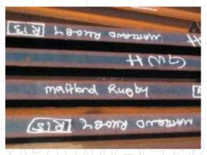
Clearly marked items make processing of loads easier for both client and galvanizer. The correct type of strippable marking paint should be use to ensure removal in the pretreatment process prior to galvanizing.
