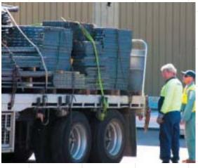
Documentation accompanying fabricated steel deliveries for galvanizing should detail all items in the consignment. The galvanizers describes and tags items after delivery to track items through the galvanizing process.
