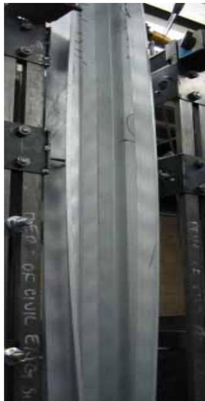
Figure 15d Interaction of buckling modes of SCR2000\_3
