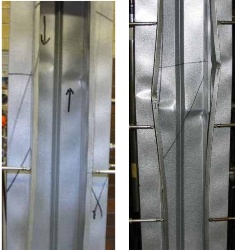
**Figure 12a & b Failure modes of SCR600\_1 (left) and SCR600\_2 (right)**
