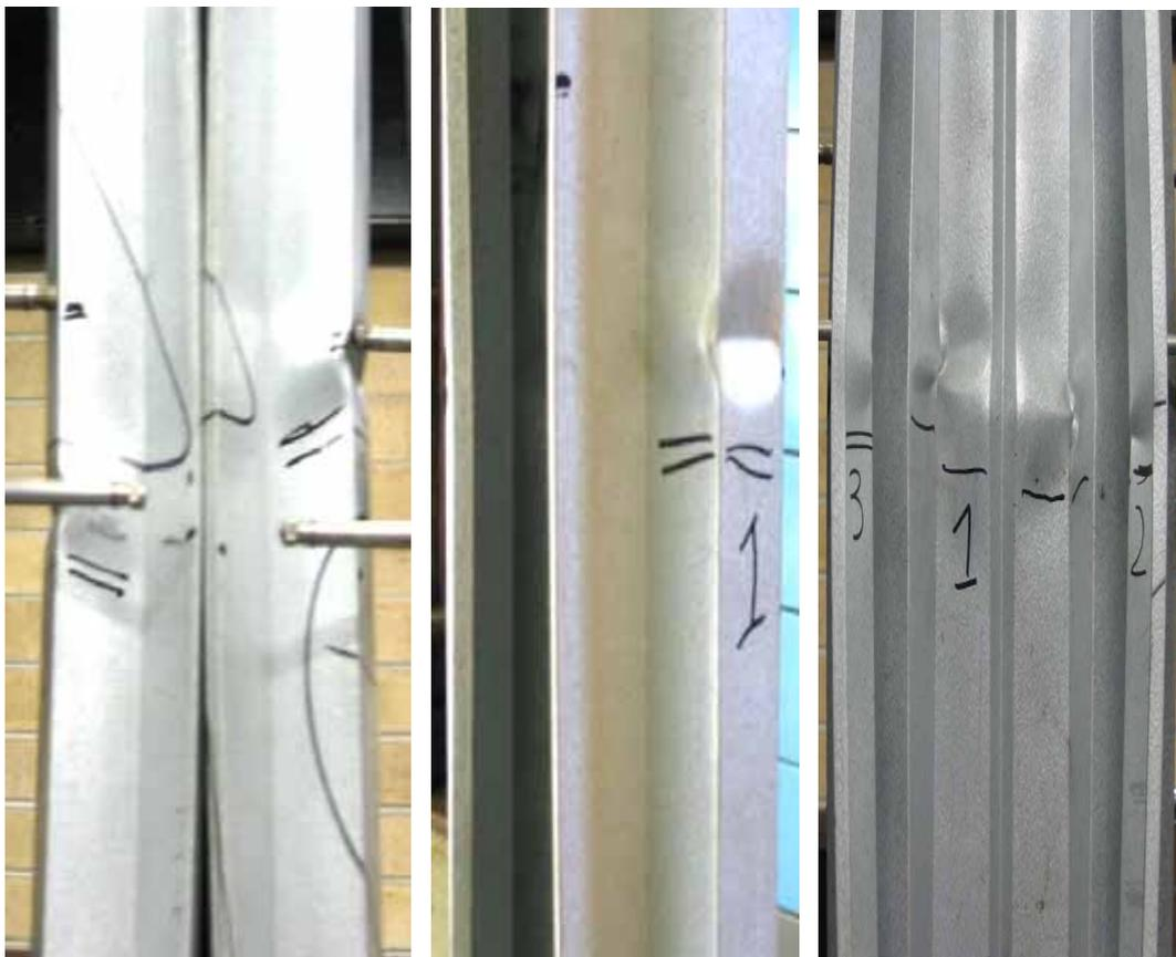
Figure 14a, b and c Failure modes of SCR1600\_1 (left), SCR1600\_2 (middle) and SCR1600\_3 (right)
