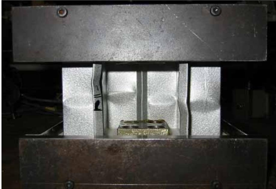
**Figure 11 Failure mode of SCR110\_2**
