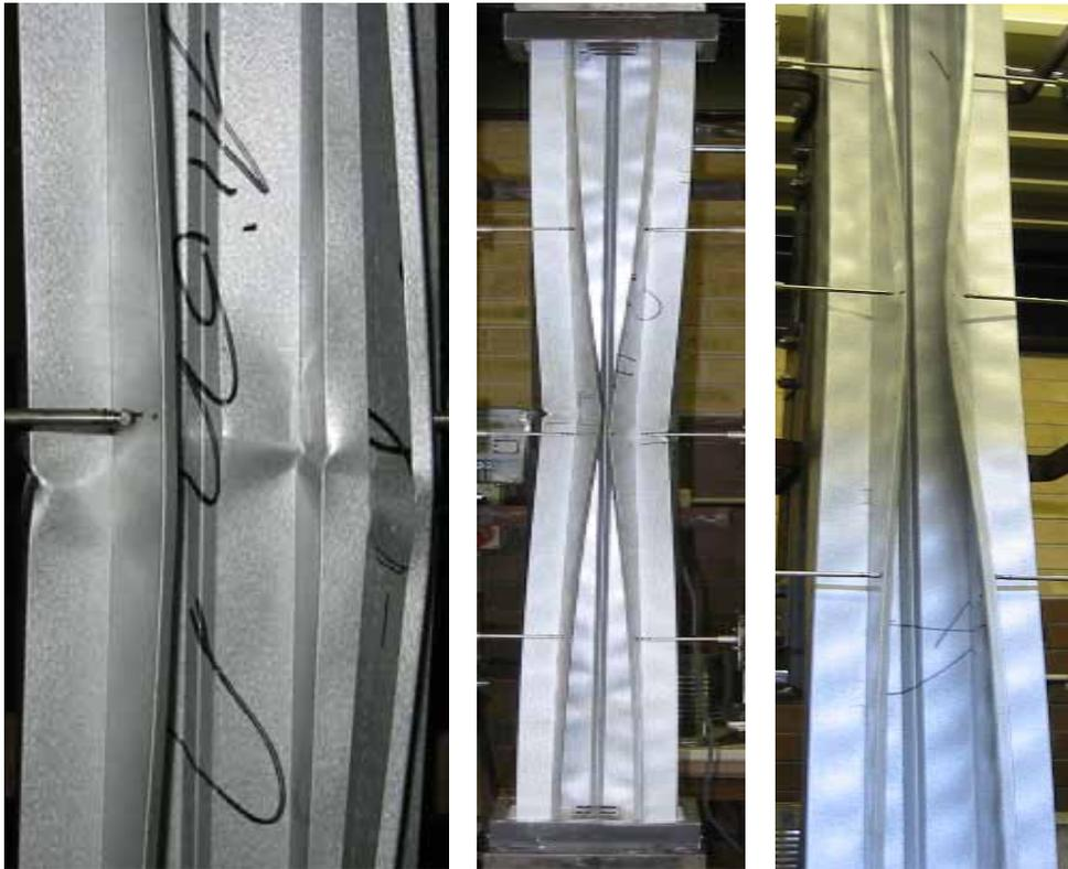
Figure 13a, b and c Failure modes for SCR1200\_1 (left), SCR1200\_2 (middle) and SCR1200\_3 (right)
