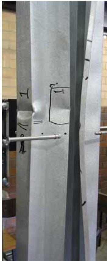
Figure 13e Failure at side flange of specimen SCR1200\_2
