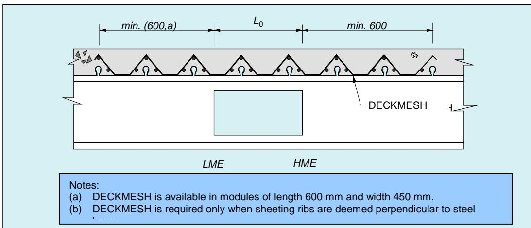
**Figure 6.2. DECKMESH™ Recommended in the Region of a Web Penetration.**
