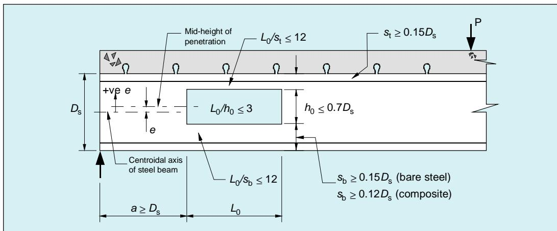
**Figure 6.1 Beam Geometry**
