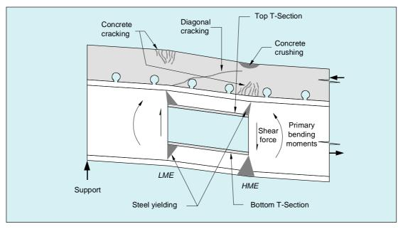
Figure 3.1 Behaviour at Ultimate Load
