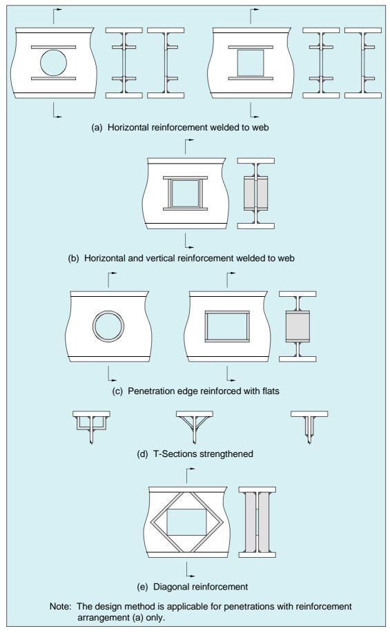
Figure 3.4 Arrangements of Web Penetration Reinforcement
