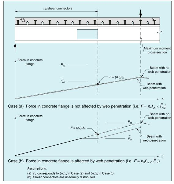
Figure 3.3 Influence of Web Penetration on Maximum Compressive Force in Concrete Flange
