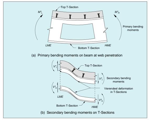
Figure 3.2 Primary and Secondary Bending Moments in the Region of a Web Penetration
