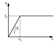
Figure 12 – Bilinear stress-strain diagram adopted for the FE material.
