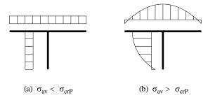
Figure 8 – Longitudinal stress distribution in T-section, a) pre-buckling stress and b) post-buckling stress.
