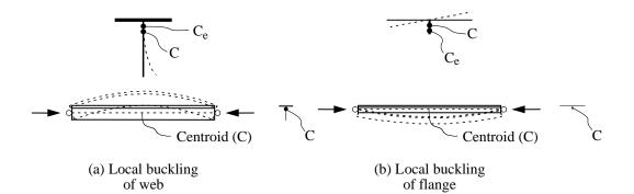
Figure 9 – Overall bending induced by the shift of the effective centroid.
