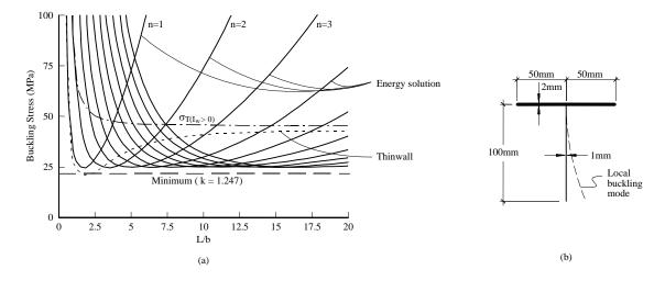
Figure 6 – Plate buckling coefficient for T-section with stocky flanges and slender web for L/b<20.
