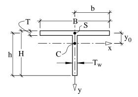
Figure 3 – Geometric definition of a T-section.
