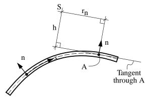
Figure 2 – Warping definition in both normal and perpendicular directions of point A.
