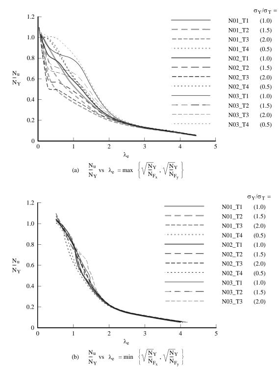
Figure 18 – Relationship between the non-dimensional failure stress/yielding stress and: a) the normalised flexural slenderness ( $\lambda_e$ ), b) the normalised global slenderness ( $\lambda_r$ ). Note: In calculating  $\lambda_r$ , the flexural-torsional buckling load includes secondary warping rigidity by determining  $I_w$  using eqn. (4).
