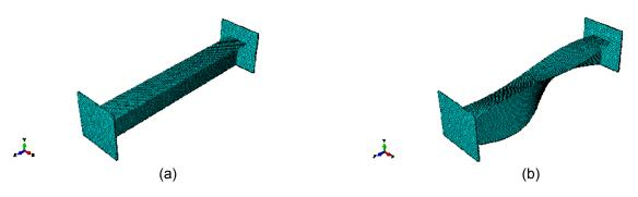
Figure 11 – Finite Element Model of Column M01\_L2, a) undeformed shape and b) deformed shape of first buckling mode.
