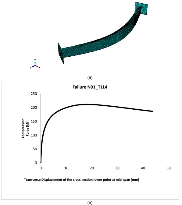
Figure 17: a) Deformed shape of Specimen N01\_T1L4 at the ultimate load (amplified 10 times); b) Forcedisplacement behaviour for specimen N01\_T1L4.
