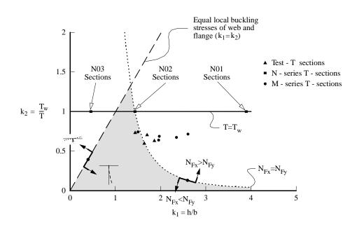
Figure  $10 - (k_1, k_2)$ -space for T-sections.
