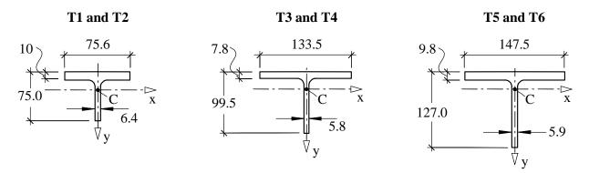
Figure 13 – Cross-section geometries of the columns tested by Kitipornchai and Lee (1986), dimensions in mm.
