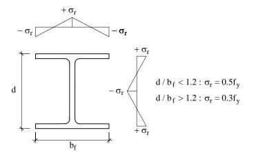
Figure 14 – Residual stresses pattern for an I-section according to ECCS (1976).
