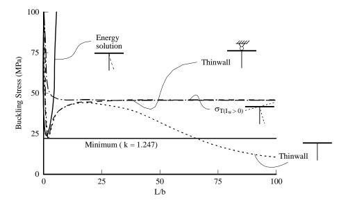
Figure 7 – Plate buckling coefficient for T-section with stocky flanges and slender web for L/b<100.
