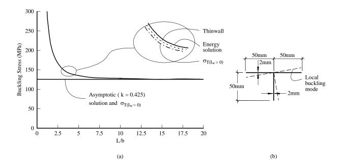
Figure 5 – Plate buckling coefficient for T-section with equal size flange and web elements.
