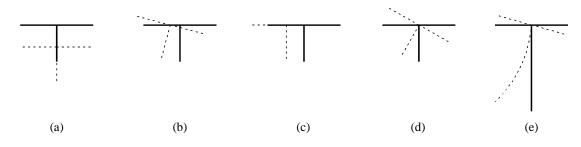
Figure 1 – Deformation modes: a) Flexural buckling in the plane of symmetry, b) Flexural-torsional buckling mode, c) Flexure about symmetry axis, d) Pure torsional and local buckling modes, and e) Local buckling modes.
