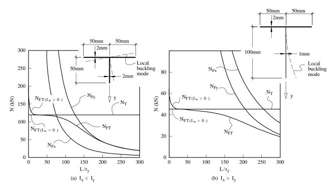
Figure 4 – Buckling load for T-sections with: a)  $I_x < I_y$  and b)  $I_x > I_y$ .
