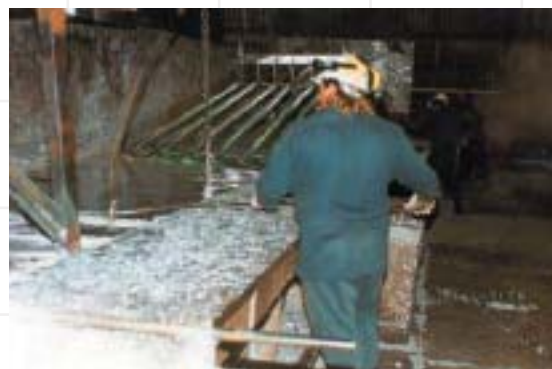
The hot dip galvanizing process involved immersion of steel fabrications in molten zinc at 455°C until the steel reaches the molten zinc temperature. Oxide residues are formed from the combined reaction between the flux, the steel and the zinc, which are here being skimmed off the surface as the work emerges from the zinc bath.
