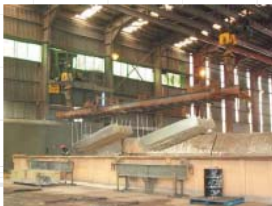
The hot dip galvanizing process involved immersion of steel fabrications in molten zinc at 455°C until the steel reaches the molten zinc temperature. Oxide residues are formed from the combined reaction between the flux, the steel and the zinc, which are here being skimmed off the surface as the work emerges from the zinc bath.
