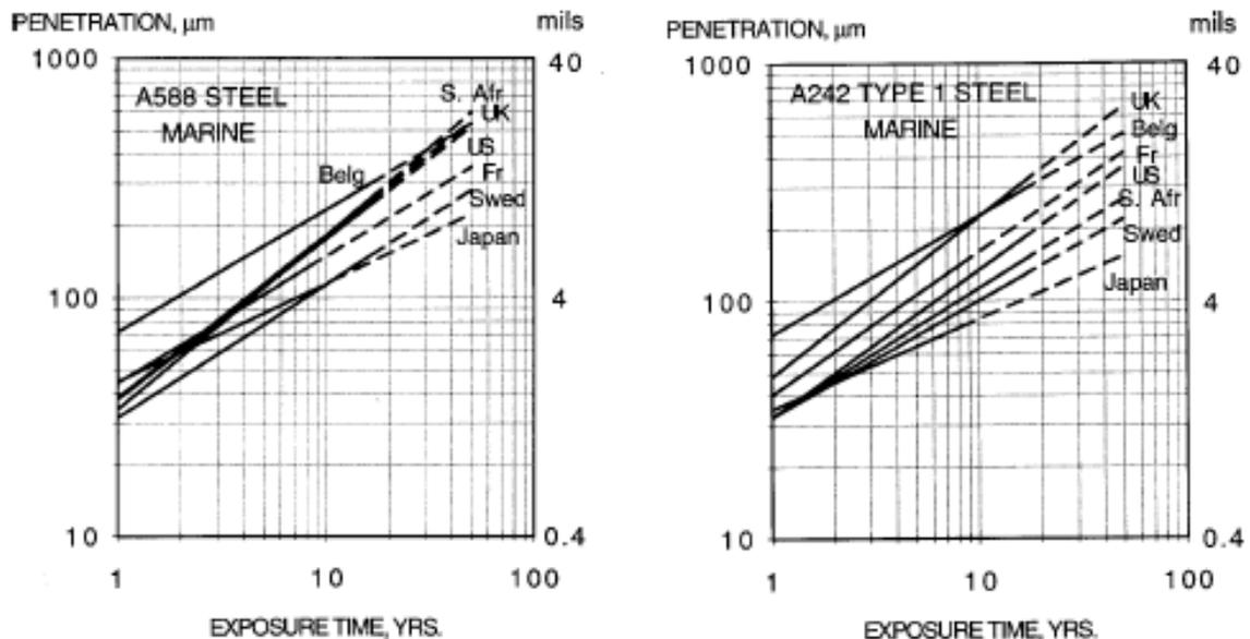
Figure 1 Projected thickness loss per surface for two weathering steel grades in a C3 marine environment [11]
