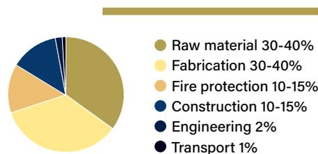
The raw material cost accounts for approximately 30% to 40% of the finished structure cost, with fabrication accounting for another 30% to 40%. Therefore, while a minimum structure weight is an admirable objective, if achieving this objective comes at the expense of overly complicated fabrication or connections, any cost saving in weight are likely to be overridden by an increased fabrication cost.
