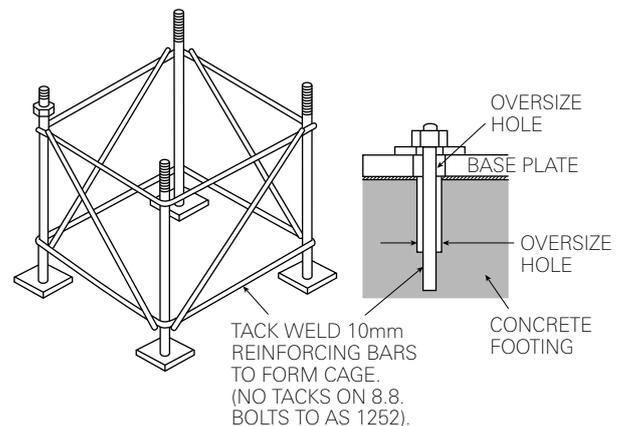
**FIGURE 8.11:** Typical holding-down bolt cage
