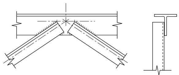
**FIGURE 8.20:** Split tee welded truss
