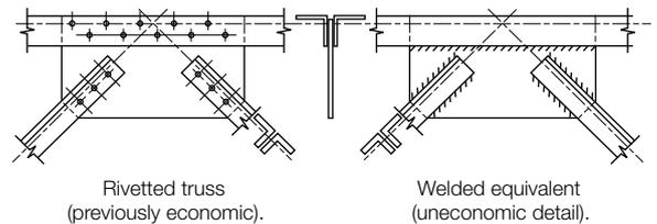
**FIGURE 8.18:** Equivalent truss detailing
