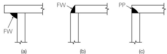
**FIGURE 8.15:** Welded corner details for box columns
