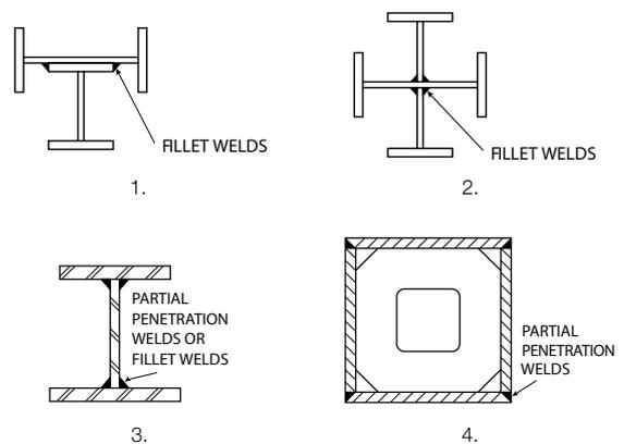
**FIGURE 8.14:** Economic details for built-up columns in ascending order of fabrication cost
