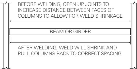
**FIGURE 8.17:** Spreading of columns to allow for weld shrinkage
