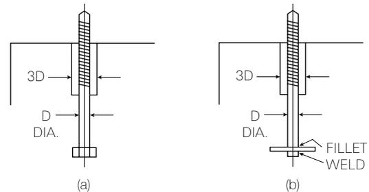
**FIGURE 8.10:** Holding-down bolt details
