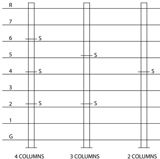
**FIGURE 8.12:** Minimise number of column splices – 1 is preferable to 3
